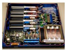
The e-OSTEO mission uses an automated minilab to carry out bone cell research in microgravity. (Photo: © Canadian Space Agency)
